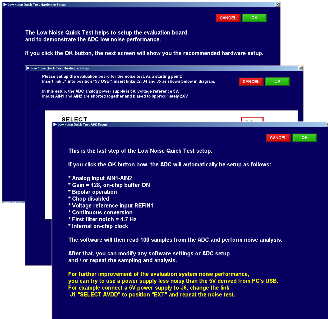
Figure 10. Low Noise Quick Test Hardware Setup
