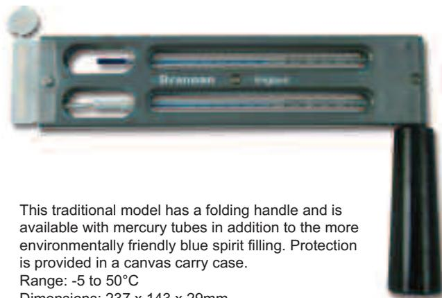
This traditional model has a folding handle and is available with mercury tubes in addition to the more environmentally friendly blue spirit filling. Protection is provided in a canvas carry case.
