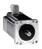
3-phase stepper motor - 6.78Nm - shaft Ø 14mm - L=128 mm - w/o brake - term box
