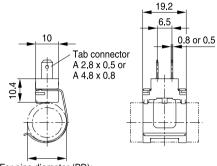
For pipe diameter (PD): ø13.5, 15, 18, 19 and 22 mm
