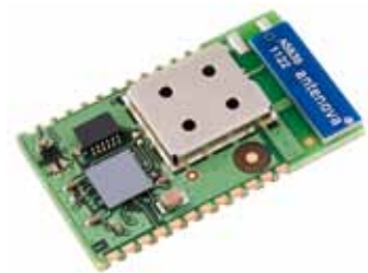
SPBT2632C1A Bluetooth® technology class-1 module
