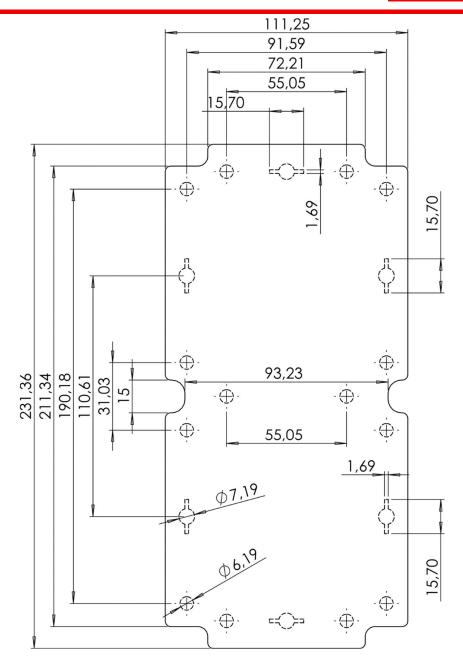
Dashed line shows outline of the mounting boss under PCB board Recommended mounting holes diameter ø2,6mm All dimensions are given within +/-0,5mm tolerance
