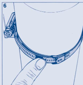
6 Push any remaining excess band through the buckle for a safe, tidy job. Tamtorque can be released and repositioned if required.
