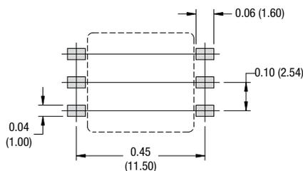
Unless otherwise stated all dimensions in inches (mm)  $\pm 0.01$  (0.25). All pins on a 0.1 (2.54) pitch and within  $\pm 0.01$  (0.25) of true position.
