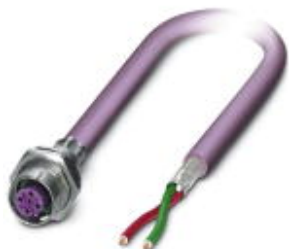
Bus system flush-type socket, PROFIBUS, 2-pos., M12, shielded, B-coded, rear/screw mounting with M16 thread, with 1 m bus cable, 2 x 0.25 mm 2
