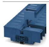
Bolt connection terminal block, Connection method: Bolt connection, Number of positions: 1, Cross section: 6 mm² - 150 mm², AWG: 10 - 300, Width: 41 mm, Color: blue, Mounting type: NS 35/7,5, NS 35/15, ct screw connection
