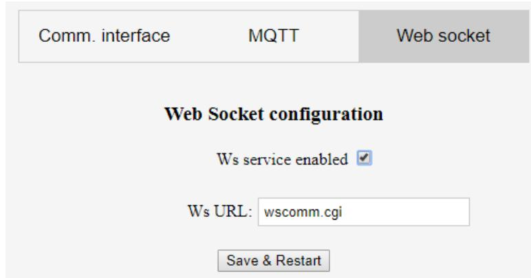
Figure 4-7 Web interface – the Web socket configuration
