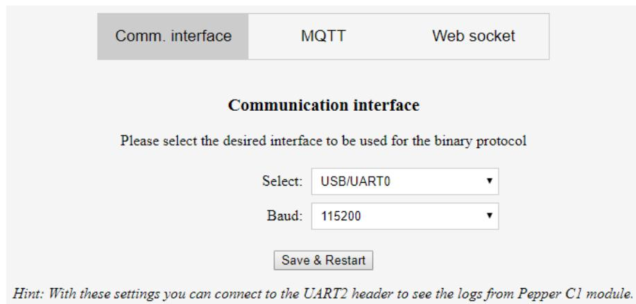
Figure 4-4 Web interface - the Communication interface tab.
