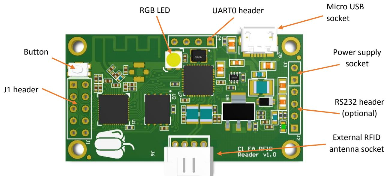
Micro USB – *only in USB version. Connected to the built in USB to TTL converter. This converter is routed to the UART0 header.*
