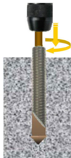
Attach setting tool to socket and spin in with drilling machine using rotary hammer action flush with surface
