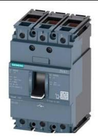
SWITCH DISCONNECTOR 3VA1 IEC FRAME 160 3-POLE SD100, IN=63A WITHOUT OVERLOAD PROTECTION WITHOUT SHORT CIRCUIT PROT. CABLE CONNECTION
