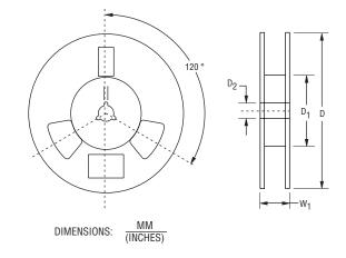
Devices are packed in accordance with EIA standard EIA-481-D and specifications shown here.
