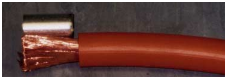
Figure 10. Showing Cable Stripped Alongside Reduction Sleeve
