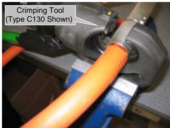
Figure 7. Example Of Crimp Operation
