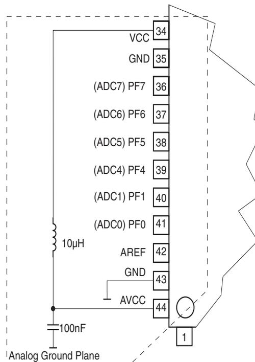
Note: The same circuitry should be used for  $AV_{CC}$  filtering on the ADC8-ADC13 side
