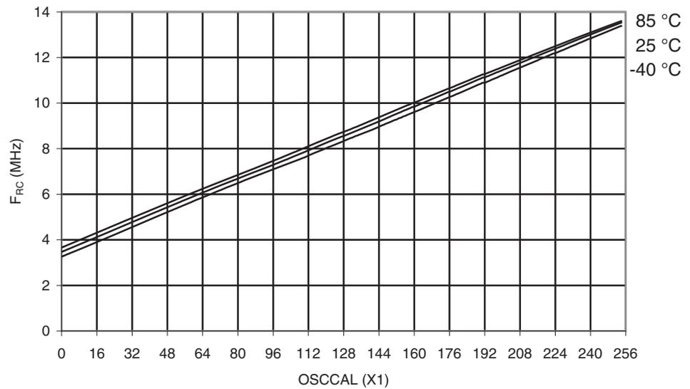
**Figure 30-36.** Calibrated 8 MHz RC Oscillator Frequency vs. Temperature
