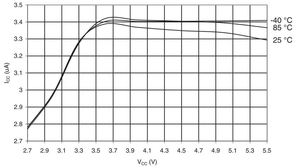
**Figure 30-40.** USB Regulator Level with load 75  $\Omega$  vs.  $V_{CC}$
