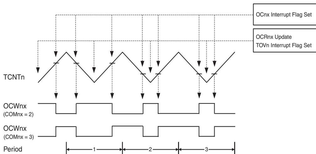
The Timer/Counter Overflow Flag (TOV4) is set each time the counter reaches BOTTOM. The Interrupt Flag can be used to generate an interrupt each time the counter reaches the BOTTOM value.
