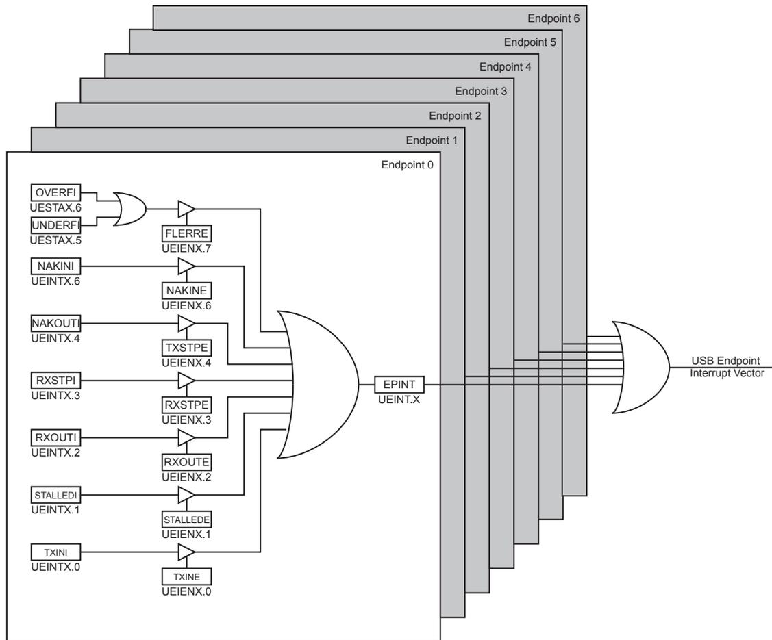
Each endpoint has 8 interrupts sources associated with flags, and each source can be enabled or not to trigger the corresponding endpoint interrupt. If, for an endpoint, at least one of the sources is enabled to trigger interrupt, the corresponding event(s) will make the program branch to the USB Endpoint Interrupt vector. The user may determine the source (endpoint) of the interrupt by reading the UEINT register, and then handle the event detected by polling the different flags.
