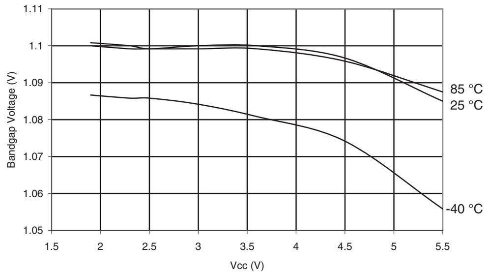
**Figure 30-32.** Bandgap Voltage vs. Temperature
