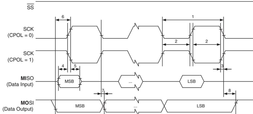
**Figure 29-5. SPI Interface Timing Requirements (Slave Mode)**
