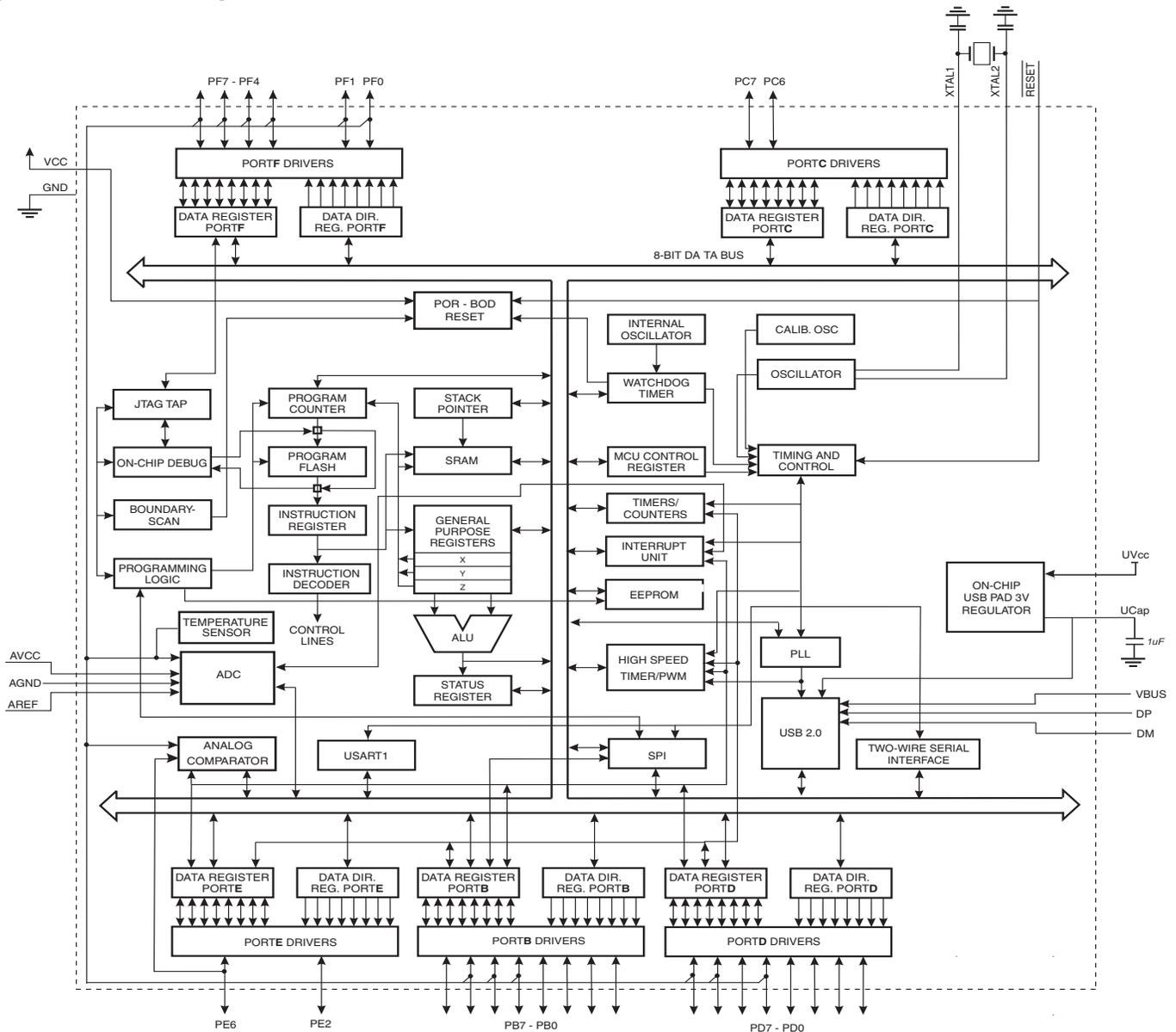
The AVR core combines a rich instruction set with 32 general purpose working registers. All the 32 registers are directly connected to the Arithmetic Logic Unit (ALU), allowing two independent registers to be accessed in one single instruction executed in one clock cycle. The resulting architecture is more code efficient while achieving throughputs up to ten times faster than conventional CISC microcontrollers.
