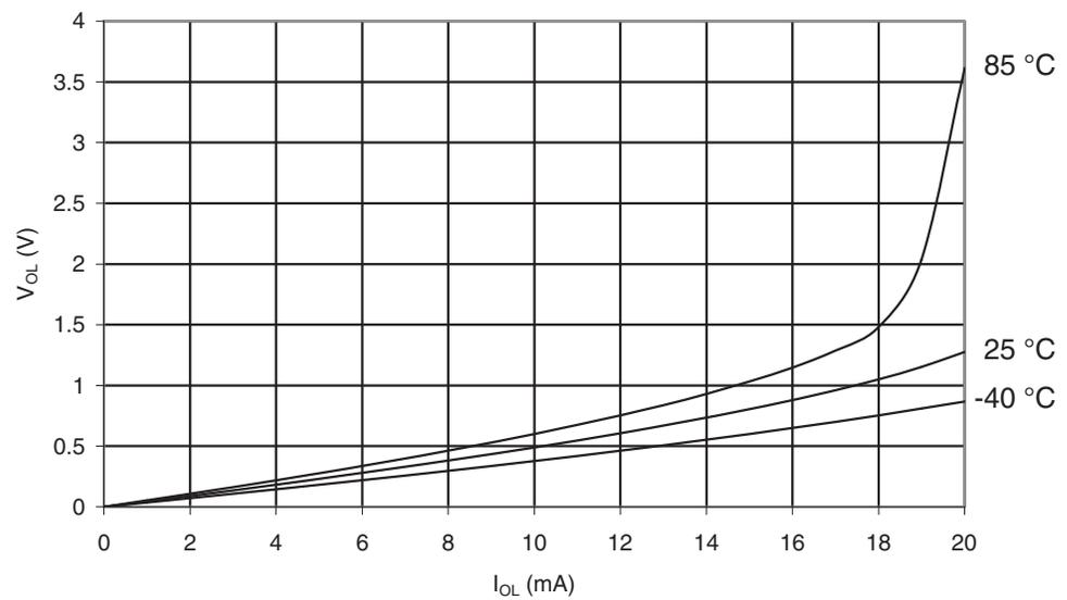
**Figure 30-18.** I/O Pin Output Voltage vs. Sink Current ( $V_{CC} = 5\text{ V}$ )
