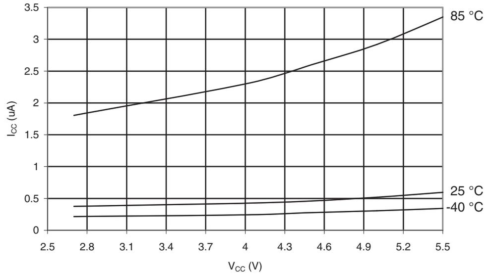
**Figure 30-11.** Power-Down Supply Current vs.  $V_{CC}$  (WDT Enabled)
