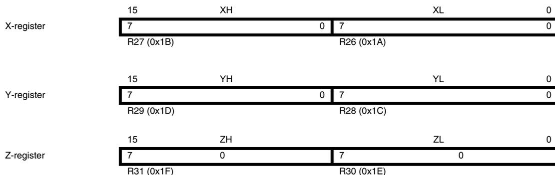
In the different addressing modes these address registers have functions as fixed displacement, automatic increment, and automatic decrement (see the instruction set reference for details).
