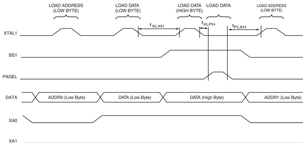
Note: 1. The timing requirements shown in Figure 28-7 (i.e.,  $t_{DVXH}$ ,  $t_{XHL}$ , and  $t_{XLDX}$ ) also apply to loading operation.
