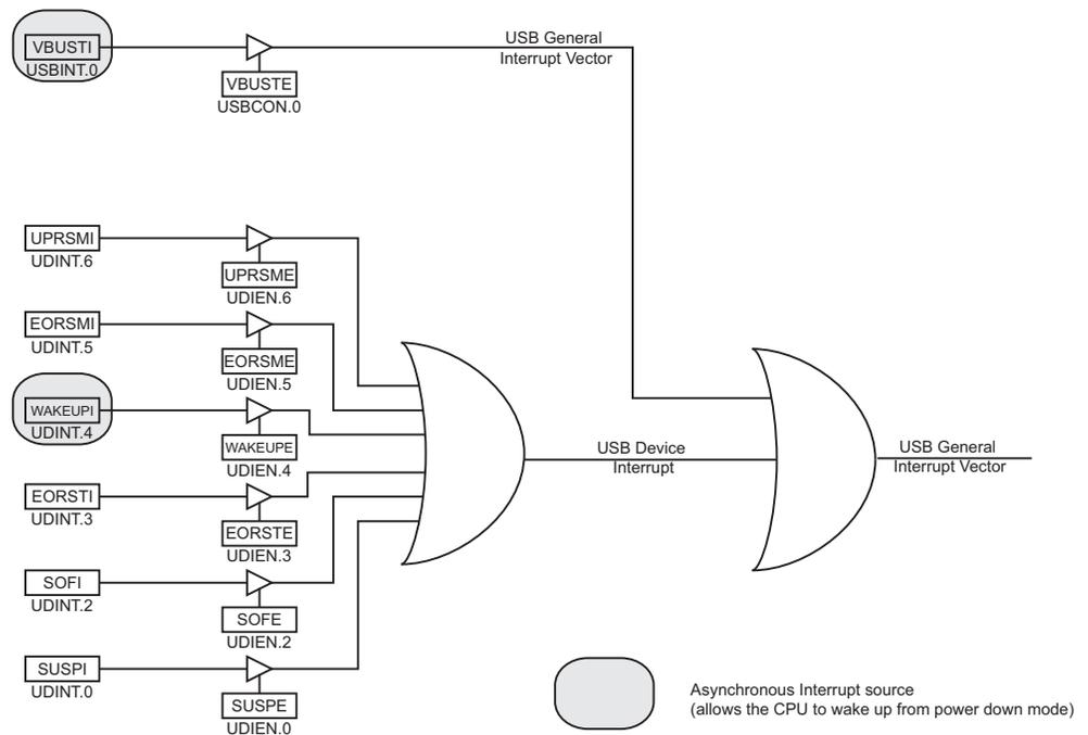
Almost all these interrupts are time-relative events that will be detected only if the USB clock is enabled (FRZCLK bit set), except for:
