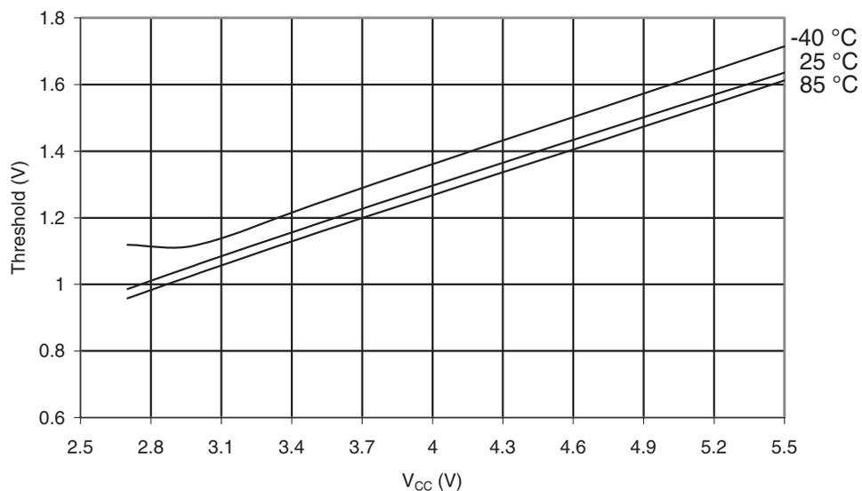
**Figure 30-24.** USB Pin Input Threshold Voltage vs.  $V_{CC}$  ( $V_{IH}$ , IO Pin read as '1')
