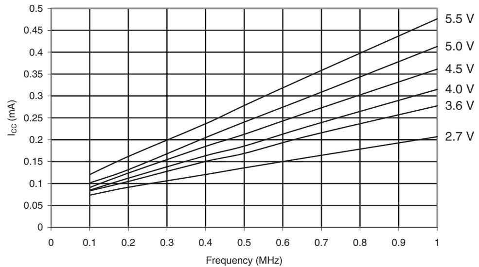
**Figure 30-8.** Idle Supply Current vs. Frequency (1-16 MHz) T = 25°C
