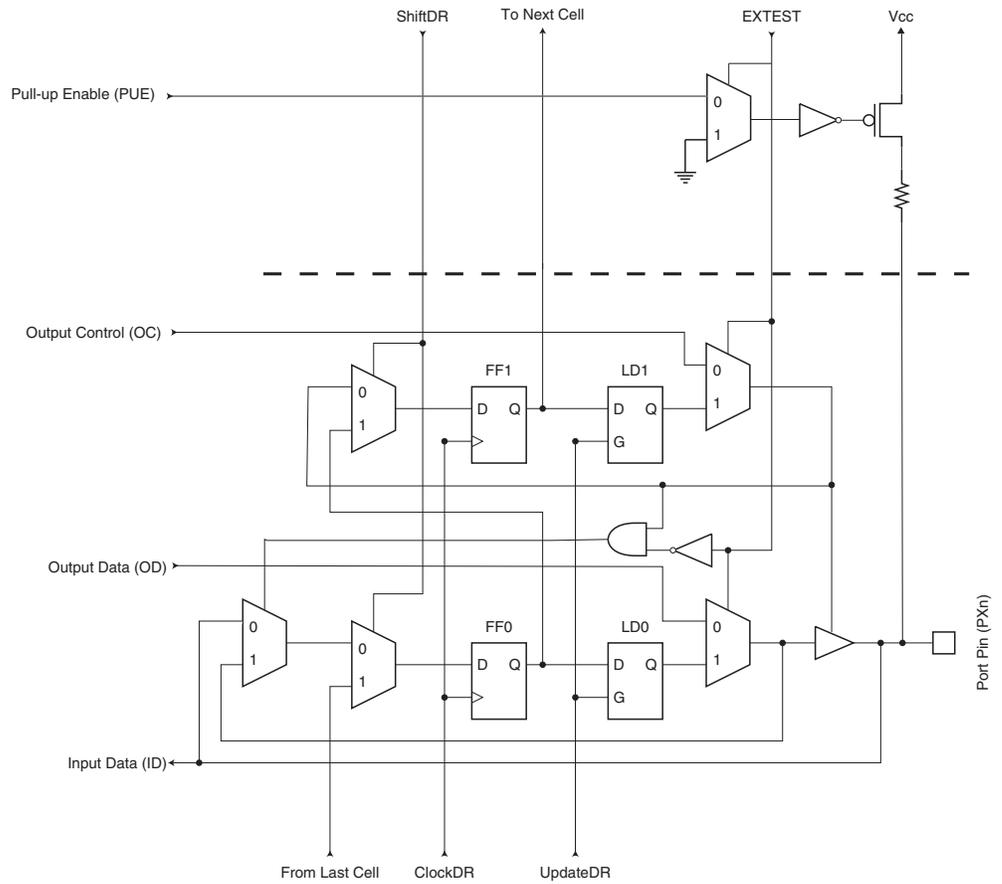
**Figure 26-4.** General Port Pin Schematic Diagram
