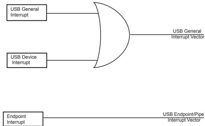
The USB hardware module distinguishes between USB General events and USB Endpoint events that are relevant with data transfers relative to each endpoint.
