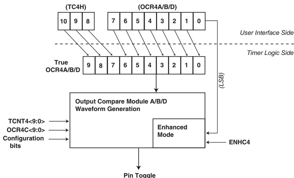
That figure shows that the true OCR4A/B/D value corresponds to the value loaded by the user shifted on the right in order to transfer the least significant bit directly to the Waveform generation module.
