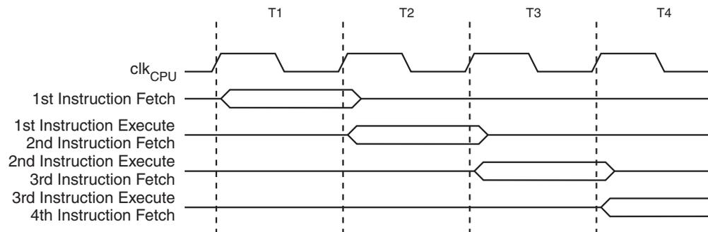
Figure 4-6 shows the internal timing concept for the Register File. In a single clock cycle an ALU operation using two register operands is executed, and the result is stored back to the destination register.
