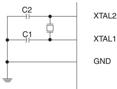
The Low Power Oscillator can operate in three different modes, each optimized for a specific frequency range. The operating mode is selected by the fuses CKSEL[3..1] as shown in [Table 6-3](#).
