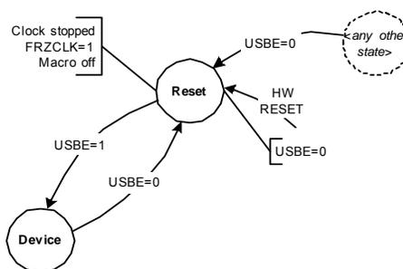
USB Controller state after an hardware reset is 'Reset'. In this state:
