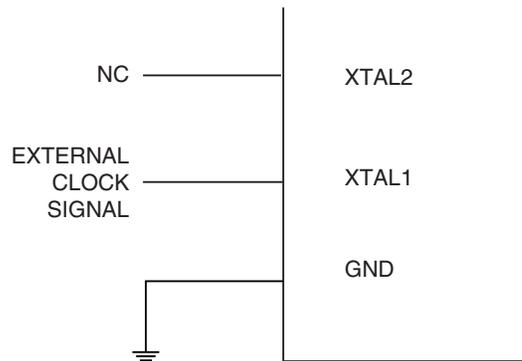
When this clock source is selected, start-up times are determined by the SUT Fuses as shown in [Table 6-9](#).
