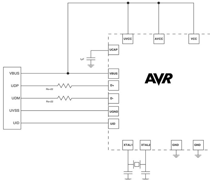
**Figure 21-4.** Typical Bus powered application with 3V I/O
