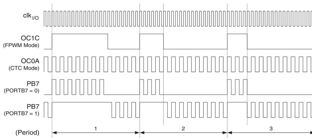
In this example, Timer/Counter0 provides the carrier, while the modulating signal is generated by the Output Compare unit C of the Timer/Counter1.
