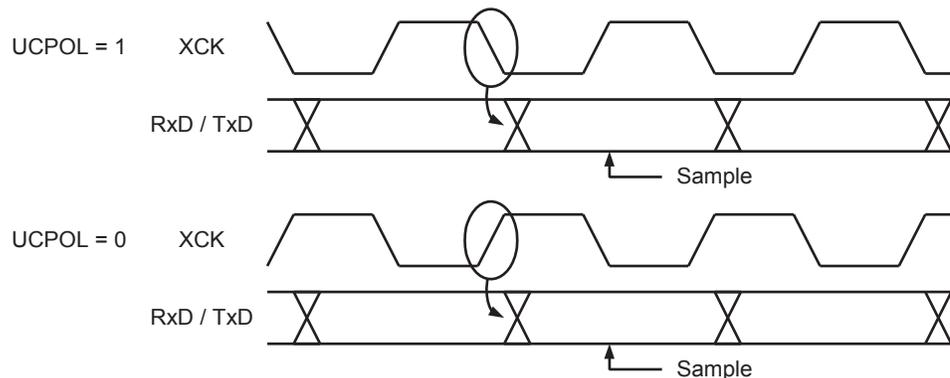
The UCPOLn bit UCRSC selects which XCKn clock edge is used for data sampling and which is used for data change. As [Figure 18-3](#) shows, when UCPOLn is zero the data will be changed at rising XCKn edge and sampled at falling XCKn edge. If UCPOLn is set, the data will be changed at falling XCKn edge and sampled at rising XCKn edge.
