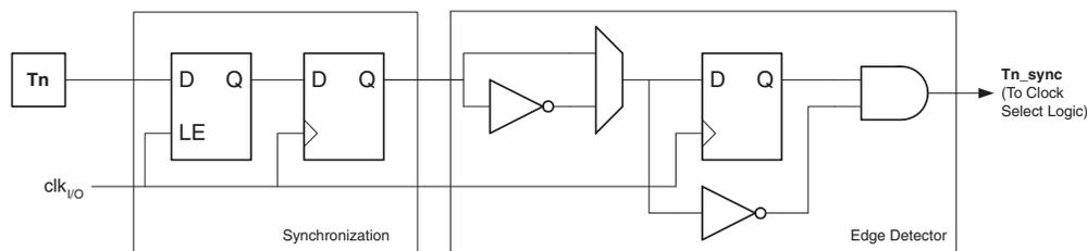
The synchronization and edge detector logic introduces a delay of 2.5 to 3.5 system clock cycles from an edge has been applied to the T<sub>n</sub> pin to the counter is updated.
