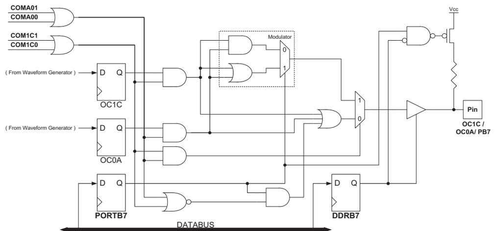
When the modulator is enabled the type of modulation (logical AND or OR) can be selected by the PORTB7 Register. When PORTB7=0, logical AND will be performed and when PORTB7=1, logical OR will be performed (see [Figure 16-3 on page 176](#)).
