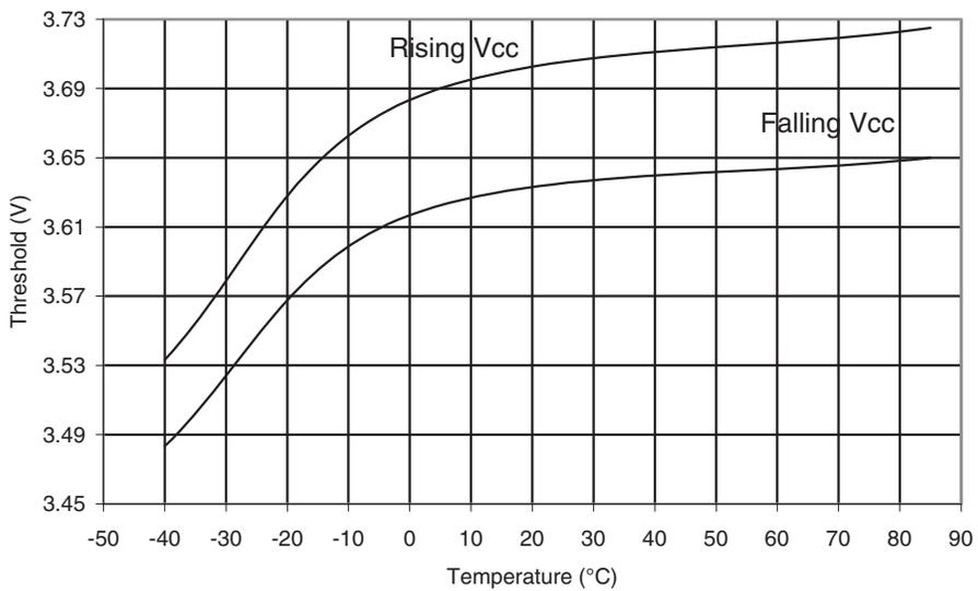
**Figure 30-30.** BOD Thresholds vs. Temperature (BODLEVEL is 4.3 V)
