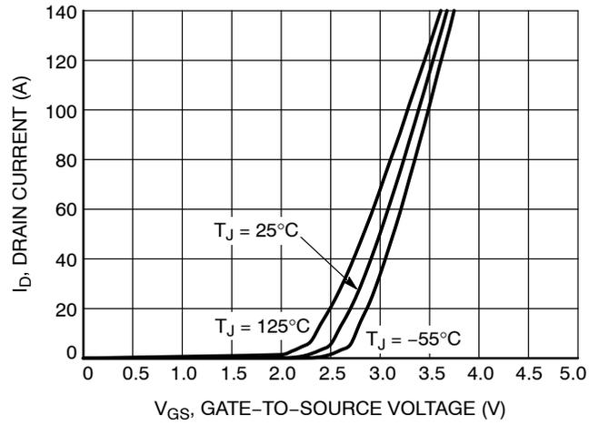
Figure 2. Transfer Characteristics
