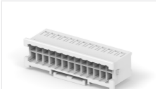
TE Part # 2-2323743-6 HOUSING, PLUG, GWT, 26P, DUAL ROW, EP2.5
