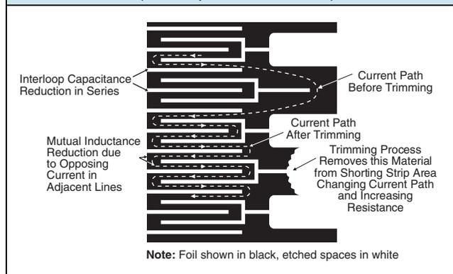
To acquire a precision resistance value, the Bulk Metal Foil chip is trimmed by selectively removing built-in “shorting bars.” To increase the resistance in known increments, marked areas are cut, producing progressively smaller increases in resistance. This method reduces the effect of “hot spot” and improves the long term stability of the hybrid chips.
