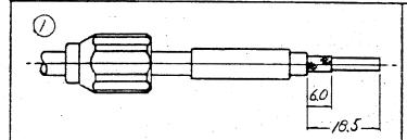
The rubber sleeve and locking nut are fitted over the cable and the outer sheath and shield are cut away as shown.
