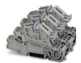
Installation ground terminal block, Spring-cage connection, cross section:  $0.08~\text{mm}^2$  -  $4~\text{mm}^2$ , AWG: 28 - 12, width: 15.6~mm, color: gray, mounting type: NS 35/7.5, NS 35/15
