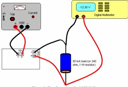
Figure 1: Test Procedure for MC34063
