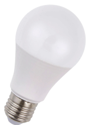
146310 LED A60 E27 95-265V AC/DC 11W (74W) 1050lm 827 Opal
