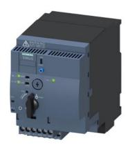
SIRIUS Compact load feeder Reversing starter 690 V 24 V AC/DC 50...60 Hz 1...4 A IP20 Connection main circuit: plug-in, without terminals Connection control circuit: screw terminal
