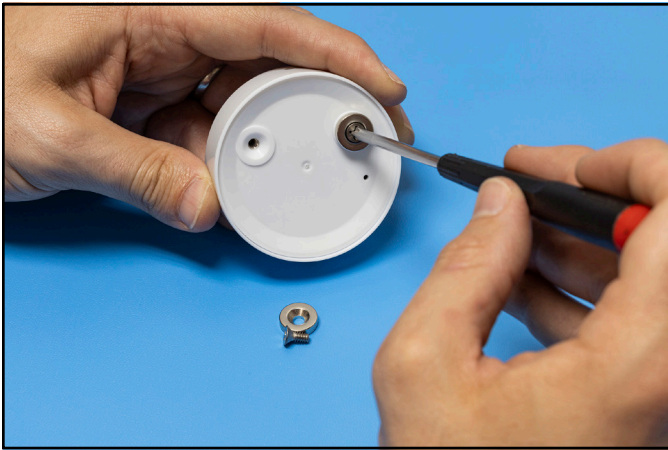
Figure 8. Installing the Desco 19344 Ring Magnets
