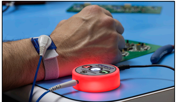
Figure 10. Illuminating red to indicate a broken operator path-to-ground
