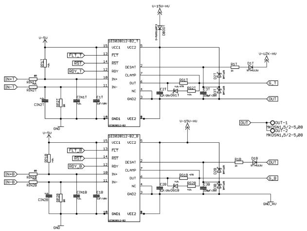
Figure 4-4 Infineon driver 1ED020I12-B2 top and bottom
