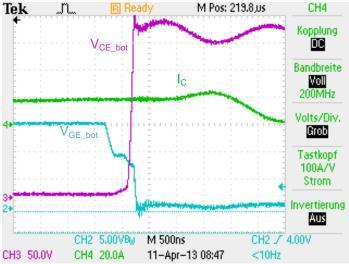
Figure 3-5 turning off bottom IGBT
