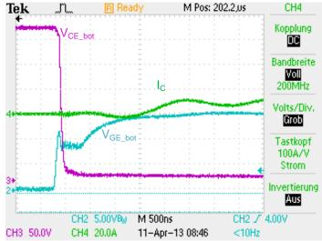
Figure 3-4 turning on bottom IGBT
