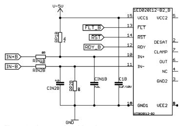
Figure 3-7 bottom side driver input
