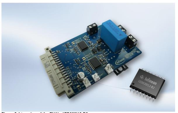
Figure 2-1 top view of the EVAL\_1ED020I12-B2
