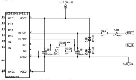
Figure 3-3 bottom side driver output
