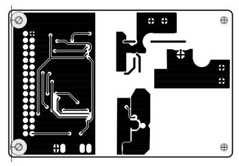
Figure 4-8 Layout bottom of the EVAL\_1ED020I12-B2
