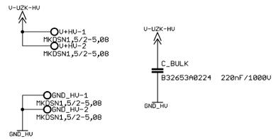
Figure 4-1 HV supply input and DC-Link
