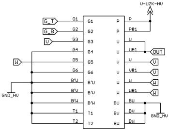
Figure 4-5 IGBT module Infineon FS25R12W1T4\_B11
