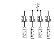
Figure 4-6 LEDs, FAULT and READY logic
