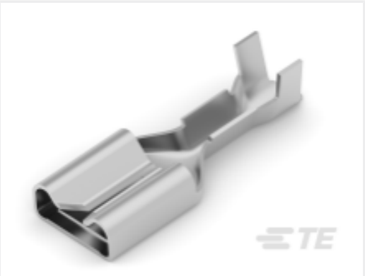
TE Part # 2238204-3 FASTON 250 STD REC STR 22-18TPBR
