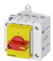
Load disconnector 3LD3, Iu 16 A Main switch 3-pole + N Rated operating capacity at AC-23 A at 400V 7.5kW Installation in distribution boards, Basic switch with selector knob red / yellow with auxiliary switch 10E + 1S
