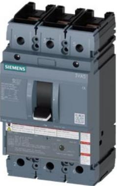
circuit breaker 3VA5 UL Frame 250 breaking capacity class H 65 kA @ 480 V 3-pole, line protection TM210, FTFM,  $In=20$  A overload protection  $Ir=20$  A permanently set short-circuit protection  $li=17.5 \times In$  UL 489 SB (naval), 50 °C, nut keeper kit on two sides
