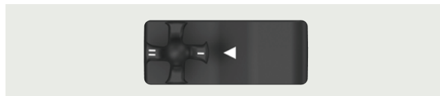
Fig. 2: Star handle for adjustment of latching force
