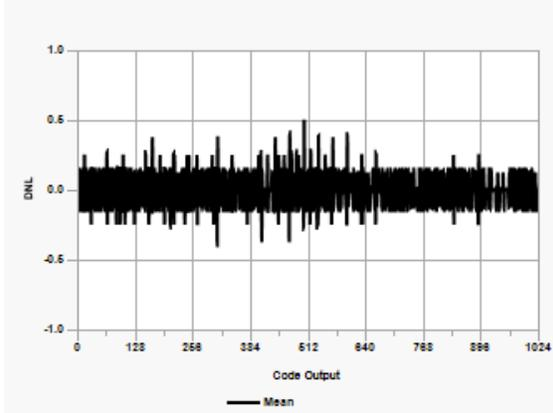
**Figure 42-2.** ADC, DNL,  $V_{DD} = 3.0V$ ,  $T_{AD} = 4 \mu s$
