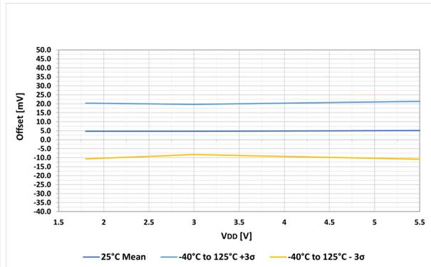
**Figure 42-15.** Comparator Common-Mode Rejection Ratio ( $V_{ICM} = V_{DD}/2$ )
