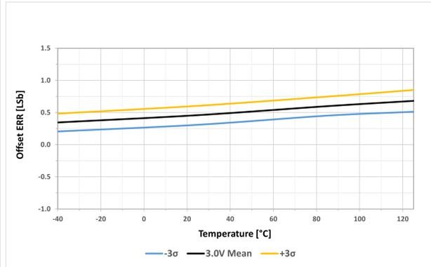
**Figure 42-20.** 8-BIT DAC, Absolute Accuracy vs. Temperature ( $V_{REF} = V_{DD} = 3.0V$ )
