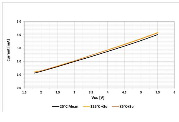
**Figure 42-33. I<sub>DD</sub>, HFINTOSC, F<sub>HFO</sub> = 32 MHz**
