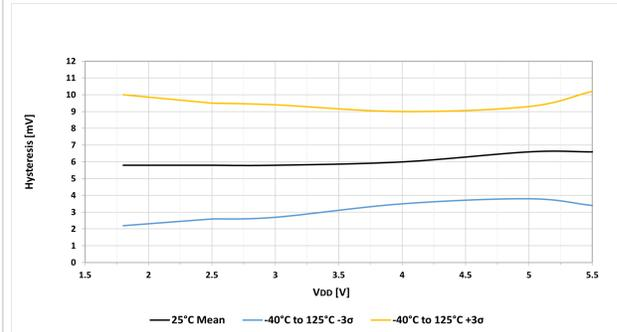
**Figure 42-14.** Comparator Offset ( $V_{ICM} = V_{DD}/2$ )
