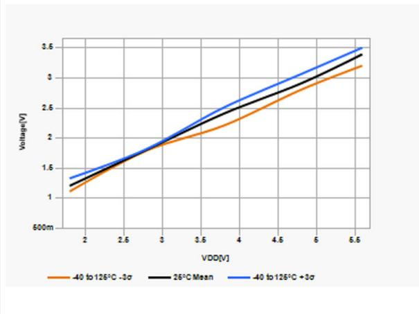
**Figure 42-35. Schmitt Trigger Low Values (V<sub>IL</sub> vs. V<sub>DD</sub>)**
