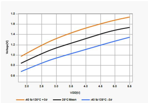
Figure 42-37. SMBus 3.0 High Value ( $V_{IH}$  vs.  $V_{DD}$ )
