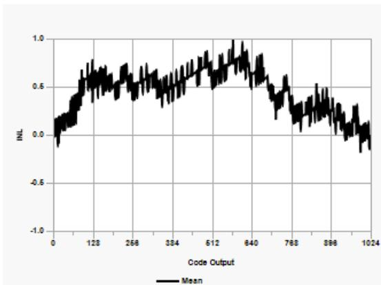
**Figure 42-6.** ADC, INL,  $V_{DD} = 3.0V$ ,  $T_{AD} = 8 \mu s$
