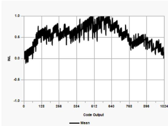
**Figure 42-5.** ADC, INL,  $V_{DD} = 3.0V$ ,  $T_{AD} = 4 \mu s$
