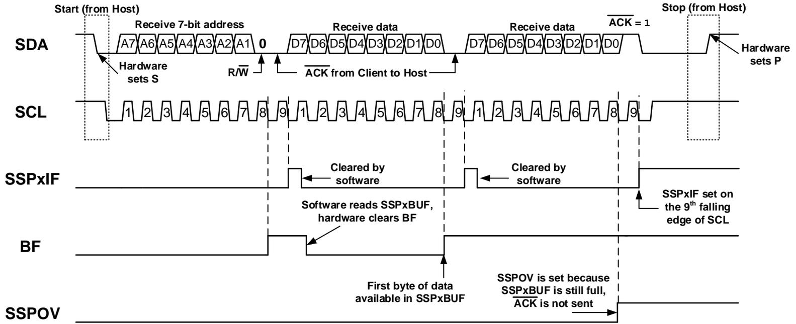
**Figure 29-16.** I<sup>2</sup>C Client, 7-Bit Address, Reception (SEN = 1, AHEN = 0, DHEN = 0)
