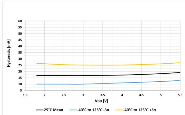
**Figure 42-13.** Comparator Hysteresis, Hysteresis Disabled ( $CxHYS = 0, V_{ICM} = V_{DD}/2$ )
