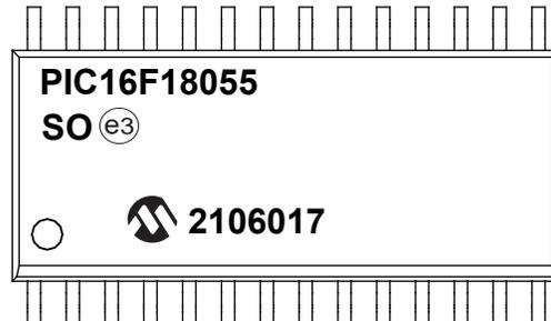
28-Lead SSOP (5.30 mm)
