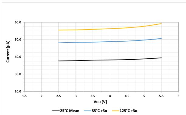
**Figure 42-45.**  $I_{PD}$ , Fixed Voltage Reference Buffer 2 (CDAFVR)
