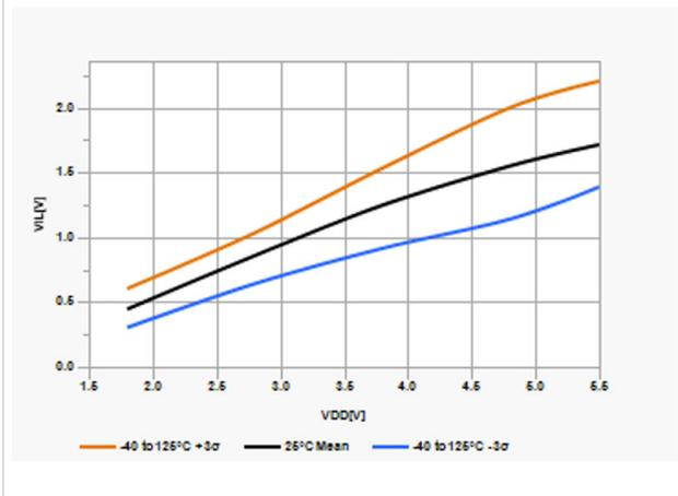
Figure 42-36. TTL Input Level
