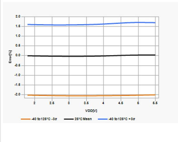
**Figure 42-26.** HFINTOSC Error % over Temperature,  $V_{DD} = 3V$
