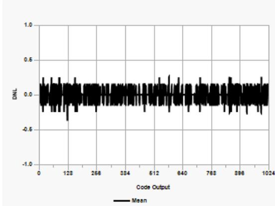
**Figure 42-3.** ADC, DNL,  $V_{DD} = 3.0V$ ,  $T_{AD} = 8 \mu s$
