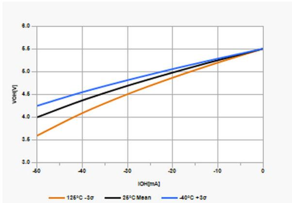
**Figure 42-53.**  $V_{OH}$  vs.  $I_{OH}$  over Temperature,  $V_{DD} = 3V$
