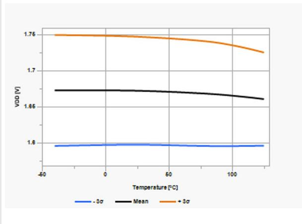
**Figure 42-51.** POR Rearm Voltage
