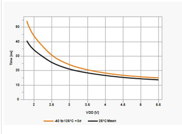
**Figure 42-30. Rise Time, Slew Rate Control Disabled**
