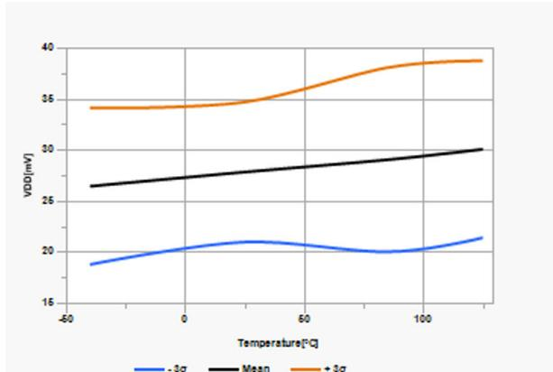
**Figure 42-9.** Brown-out Reset Voltage, Trip Point (BORV = 1)
