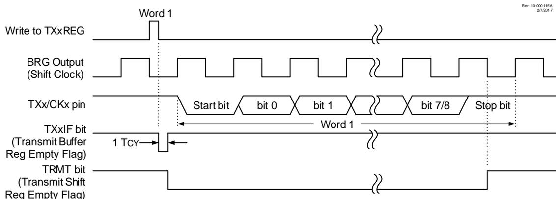
**Figure 30-4.** Asynchronous Transmission (Back-to-Back)
