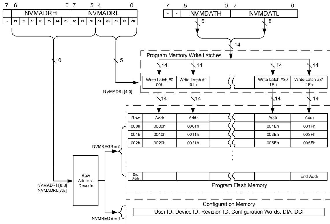
Figure 15-5. Program Flash Memory Write Sequence
