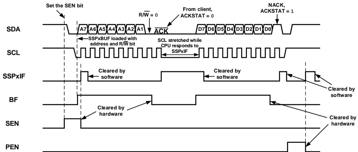
Figure 29-30. I<sup>2</sup>C Host Mode Waveform (Transmission, 10-Bit Address)
