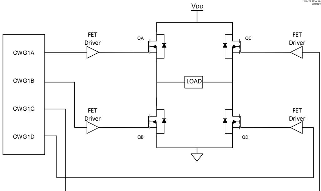
Figure 23-6. Simplified CWG Block Diagram (Forward and Reverse Full Bridge Modes)
