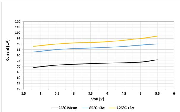
**Figure 42-44.**  $I_{PD}$ , Fixed Voltage Reference Buffer 1 (ADFVR)
