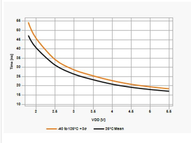
**Figure 42-29.** Fall Time, Slew Rate Control Enabled
