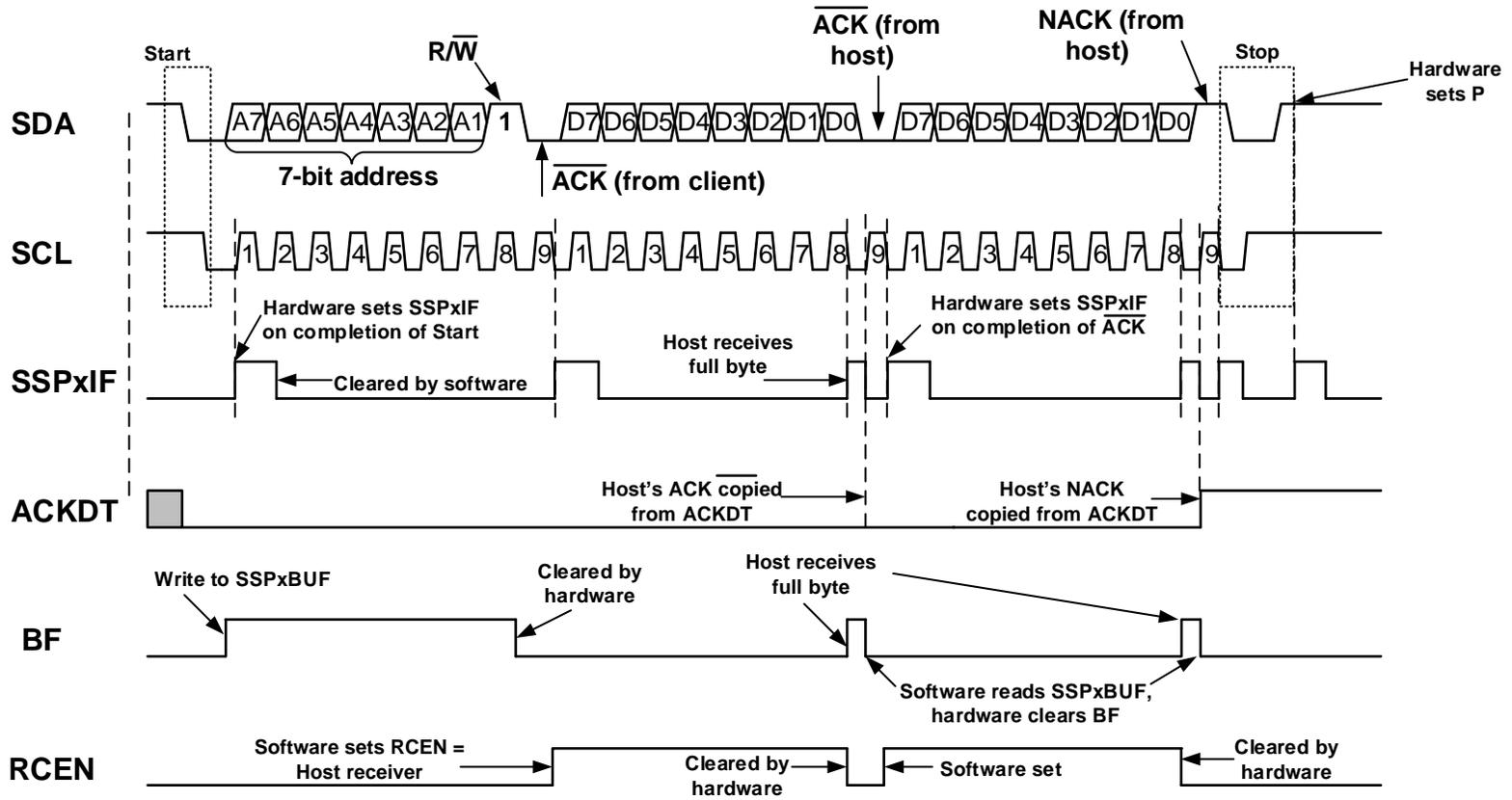
Figure 29-32. I<sup>2</sup>C Host Mode Waveform (Reception, 10-Bit Address)
