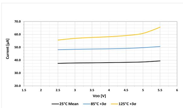
**Figure 42-46.**  $I_{PD}$  Secondary Oscillator (SOSC)
