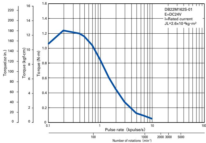
The data are measured under the drive condition of our company. The drive torque may vary depending on the accuracy of customer-side equipment.
