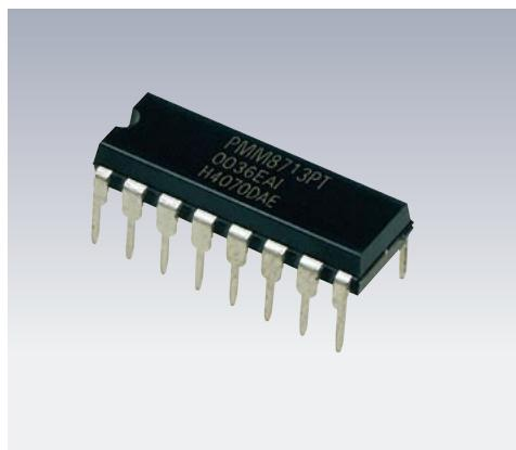
Universal controller IC for the 2-phase stepping motor drive
