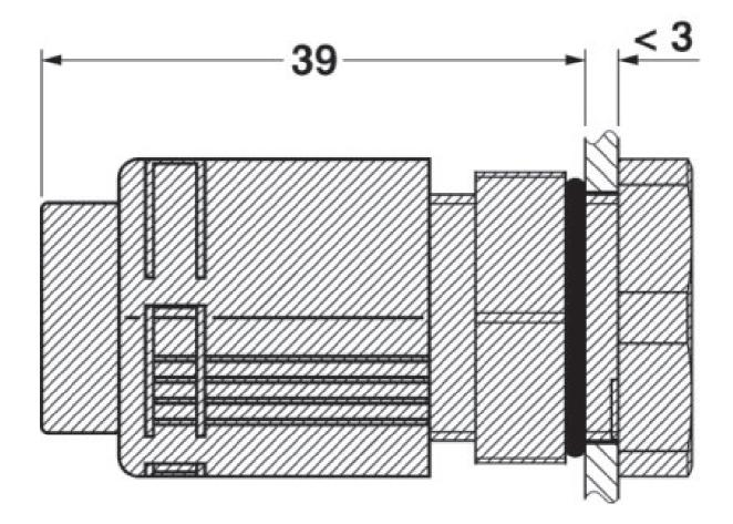
QUICKON panel feed-through with Q-SMU PG 13,5 safety nut, locked with Q-MU PG 13,5 counter nut.
