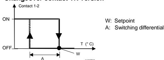
If the probe has cooled down to a temperature below approx.  $-20^{\circ}\text{C}$ , the control current circuit opens, however, automatically closes again, when the temperature rises.
