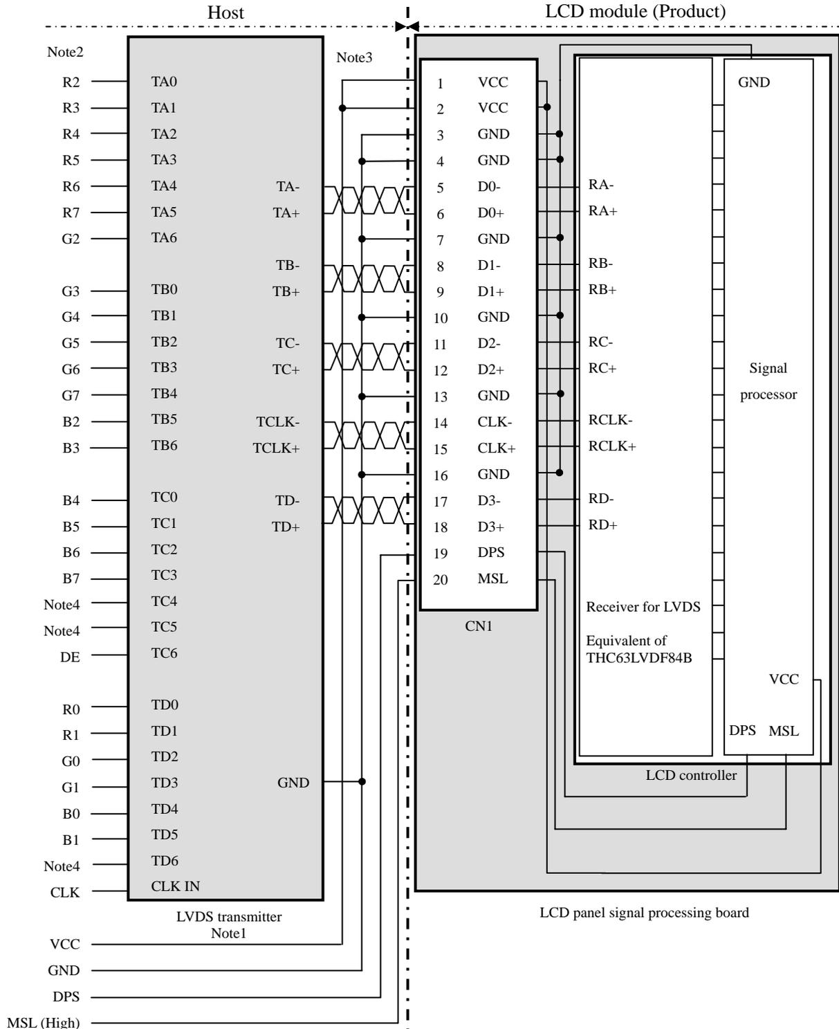
Note1: Recommended transmitter: THC63LVDM83R (THine Electronics Inc.) or equivalent
