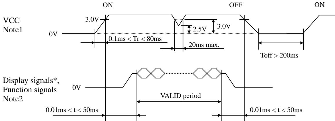
\* These signals should be measured at the terminal of 100Ω resistance.
