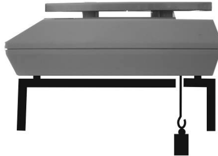
Fig. 1: Setup of balance for underfloor weighing
