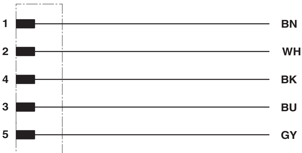
Contact assignment of the M12 plug
