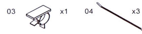
Use cable holder 03 & cable tie 04 supplied to finish cable management.
