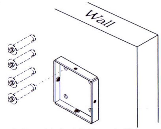
Secure bottom plate firmly to the wall with four expansion screws (not supplied).
