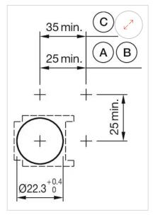
A = Solder/Plug-in terminal 2.8 mm x 0.5
