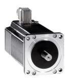
3-phase stepper motor - 6.78 Nm - shaft Ø 14mm - L=128mm - w/o brake - conn
