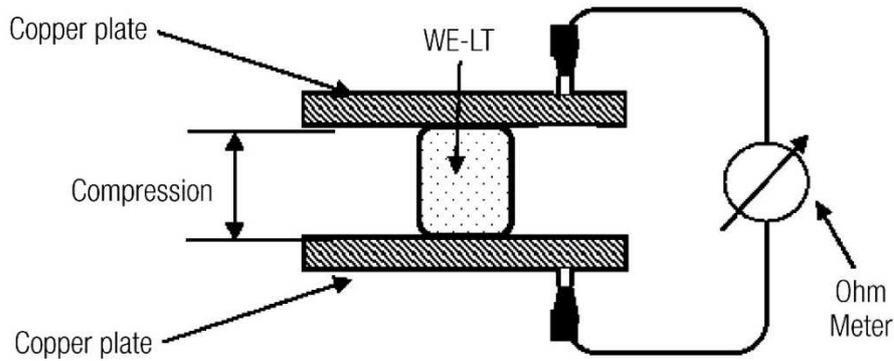
Fig. 4: Test setup surface resistance WE-LT vs. compression
