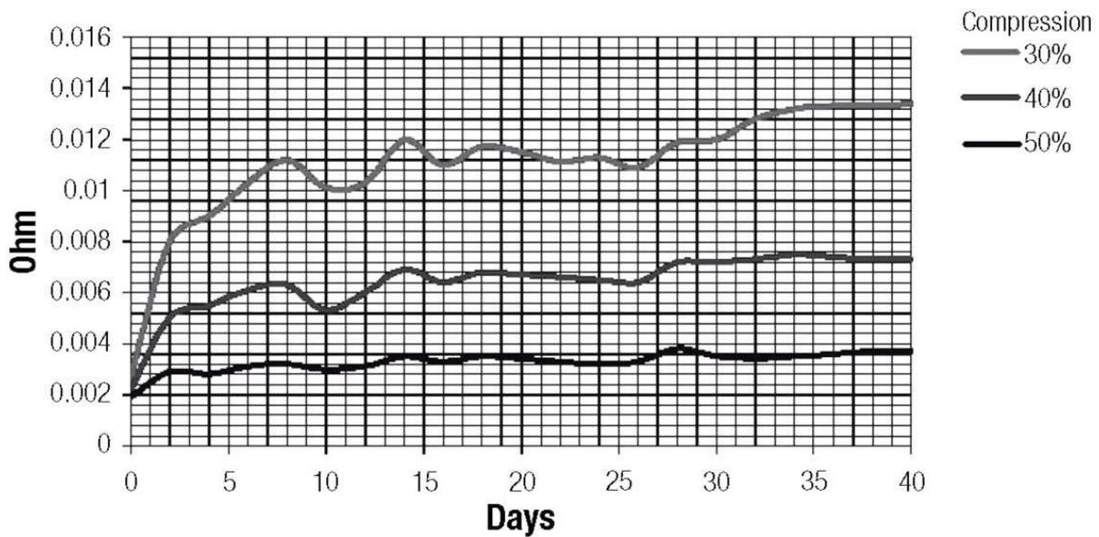
Fig. 5: Long-term run surface resistance vs. compression
