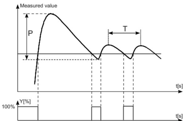
*Fig.12. Selection of settings by the oscillation method.*
