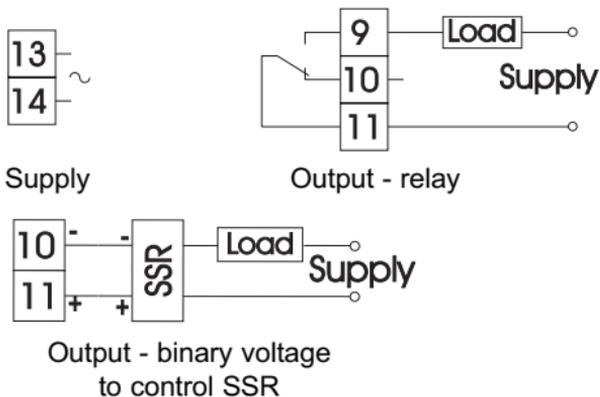
*Fig.5. Connection of the supply and load circuit.*
