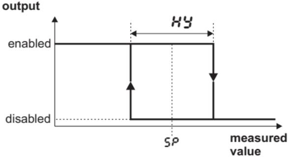
Fig.10. Operation way of the heating type output
