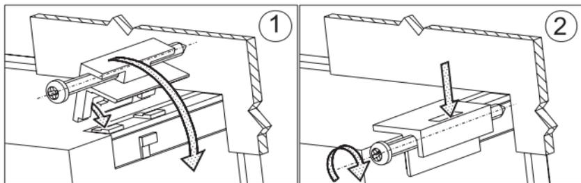
*Fig.1. Controller fixing.*
