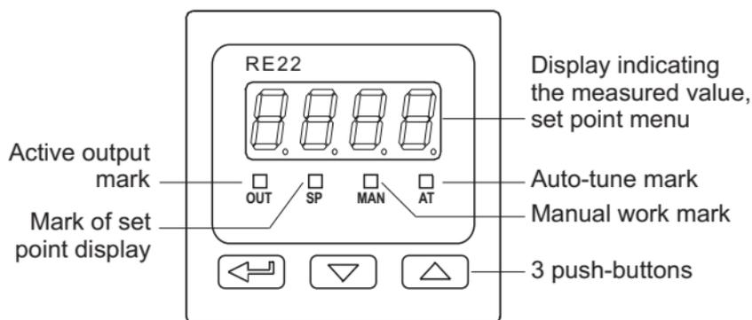
*Fig.6. View of the controller frontal plate.*
