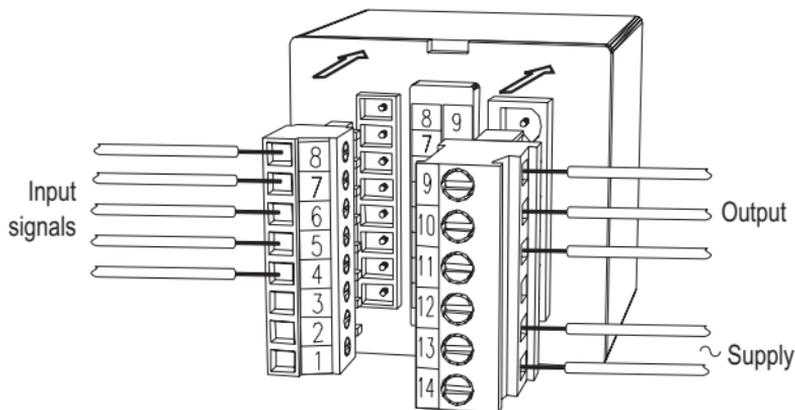
Fig.3. View of controller connection strips.
