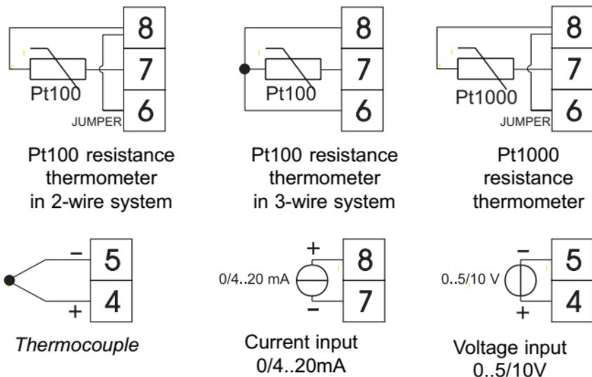
Fig.4. Connection of input signals.
