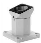
Turning range of 300 degrees. Enclosure is mounted at a 15-degree incline angle. Cast aluminum finished in RAL 7035 light-gray polyester powder paint. Setscrews and gaskets are included. Mounting fasteners are not provided.
