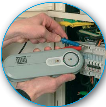
The DT-500 can bypass the phase and neutral in order to protect sensitive equipment (electronics, computers, etc.).
