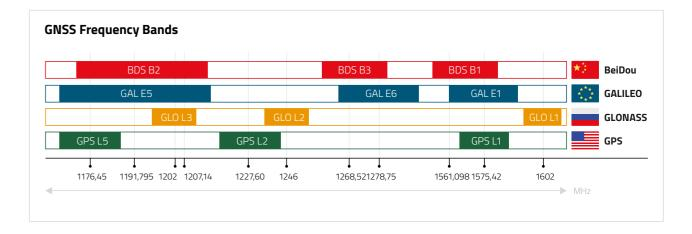
Signals from the different constellations can coexist on the same frequency bands. Each GNSS provides different signals and services over these frequency bands with different access policies. For example, open signals on the L1 frequency band are mostly used for civil commercial applications.
