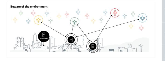
The application environment of the receiver plays an important role in the navigation, with best performance obtained in open-sky conditions. Presence of obstacles and multipath effects define a GNSS challenging environment (e.g. urban canyons), where the receiver has to work with fewer and weaker signals. This makes multi-GNSS even more decisive to the receiver's performance, since more satellites are available for tracking in a given area.
