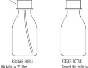
Connect this bottle to Pump Riser Hold upside down. Then squeeze and release to bleed system
