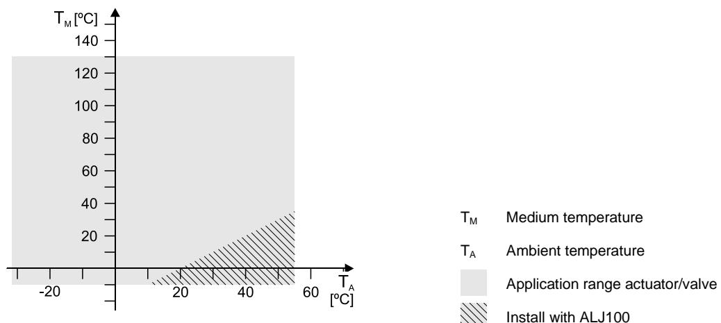
Use GDB.., GSD.., GQD.. and GDD.. actuators only at medium temperatures  $> 0$  °C.
