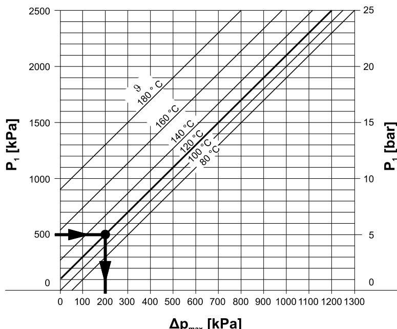
$\Delta p_{max}$  = Differential pressure at a nearly closed ball valve to largely avoid cavitation
