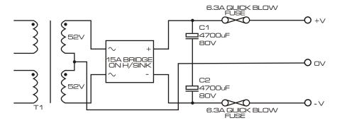
T1 = 250VA 52-0, 52-0 C1/C2 = 4700uF 80V ELECTROLYTICS BRIDGE = 15A 400V PIV THE MAINS INPUT PRIMARY MUST BE PROTECTED BY A HBC CERAMIC FUSE. A 6.3A RATING IS SUGGESTED.
