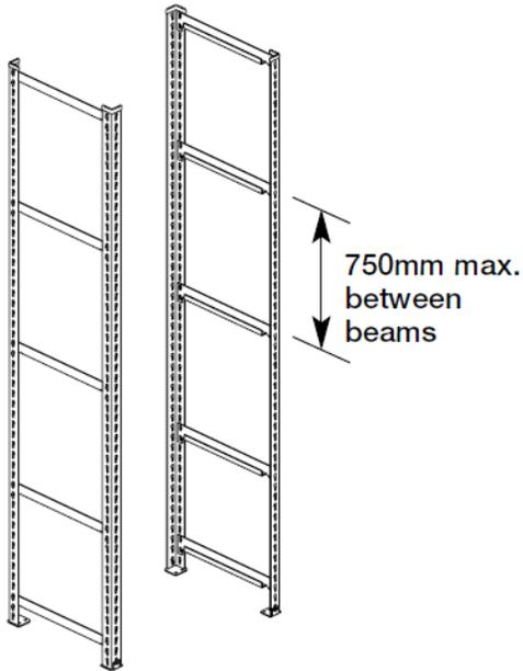
Locate mid-shelf long beams to first side frame, then to second frame.
