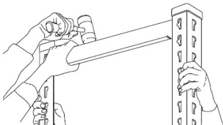
Note: Downward pointing triangular slot indicates direction for correct location
