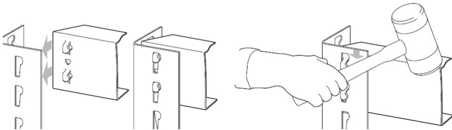
Locate top short beam, position at highest shelf position required.
