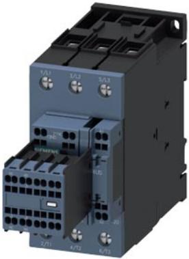
power contactor, AC-3e/AC-3, 41 A, 18.5 kW / 400 V, 3-pole, 48-80 V AC/DC, 50/60 Hz, with integrated varistor, auxiliary contacts: 2 NO + 2 NC, main circuit: screw terminal, control and auxiliary circuit: spring-loaded terminal, size: S2, removable auxiliary switch
